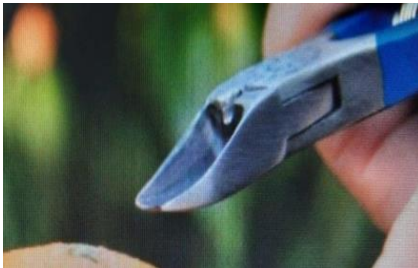
Figure 2: Good clippers with short, rounded blades and a rounded tip. This type of clippers allows a close, safe cut even when being used above the picker's head.
