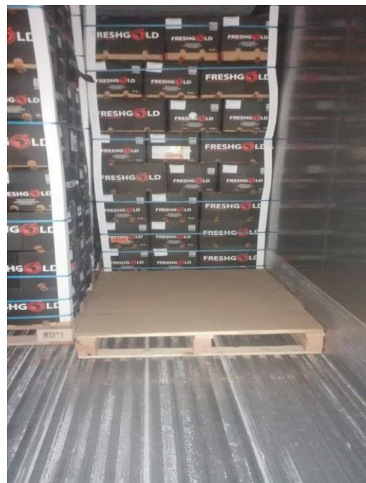
Figure 3: Examples of a wooden base with corrugated carton and airbags. Note that one piece of undamaged corrugated carton has been placed onto the top the pallet base.
