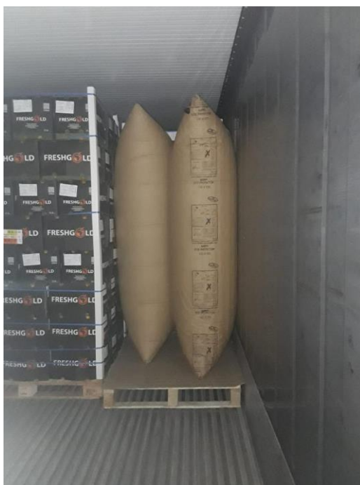
Figure 3: Examples of a wooden base with corrugated carton and airbags. Note that one piece of undamaged corrugated carton has been placed onto the top the pallet base.
