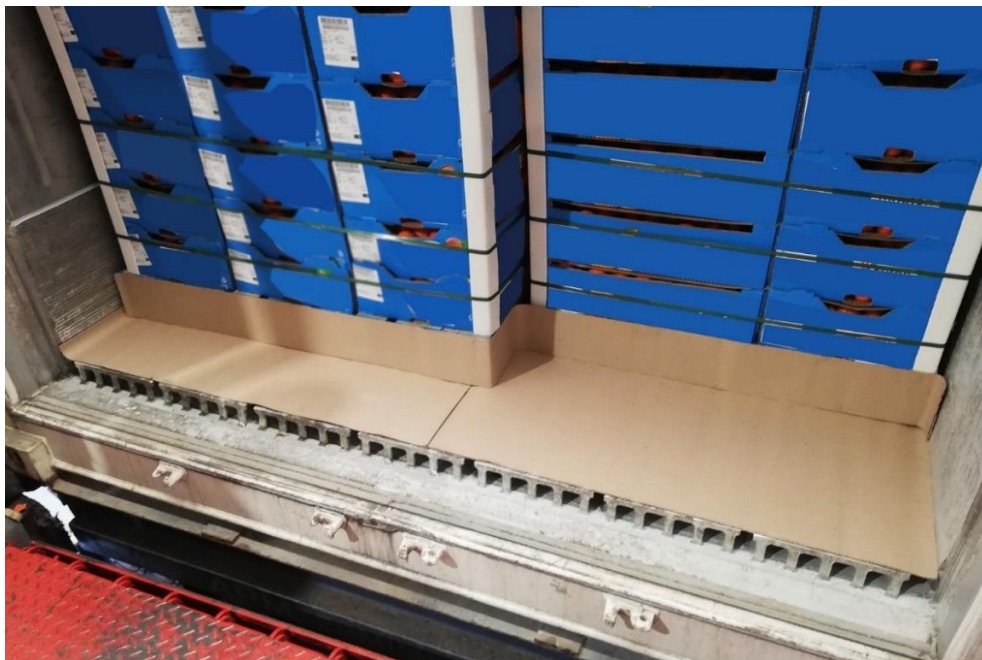
Figure 1: A correctly installed void plug. Note: (1) The void plug stops at the end of the T-bar floor. (2) All openings along the floor and pallet bases have been closed. (3) There is no chance of the void plug moving or folding up during the voyage.
