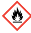
Flammable substances Self reactive substances Pyrophoric substances Self heating substances Substances emit flammable gases Organic peroxides
