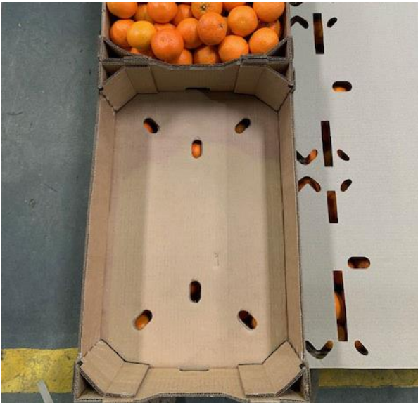
Figure 2: Illustrates how the vent holes at the bottom of the Opentop cartons must align with the holes in the securing sheet.
